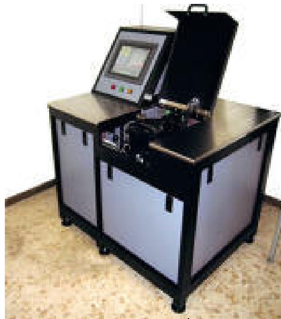
IsoVac Radiflo Mark VI Kr-85 leakage Test Machine
