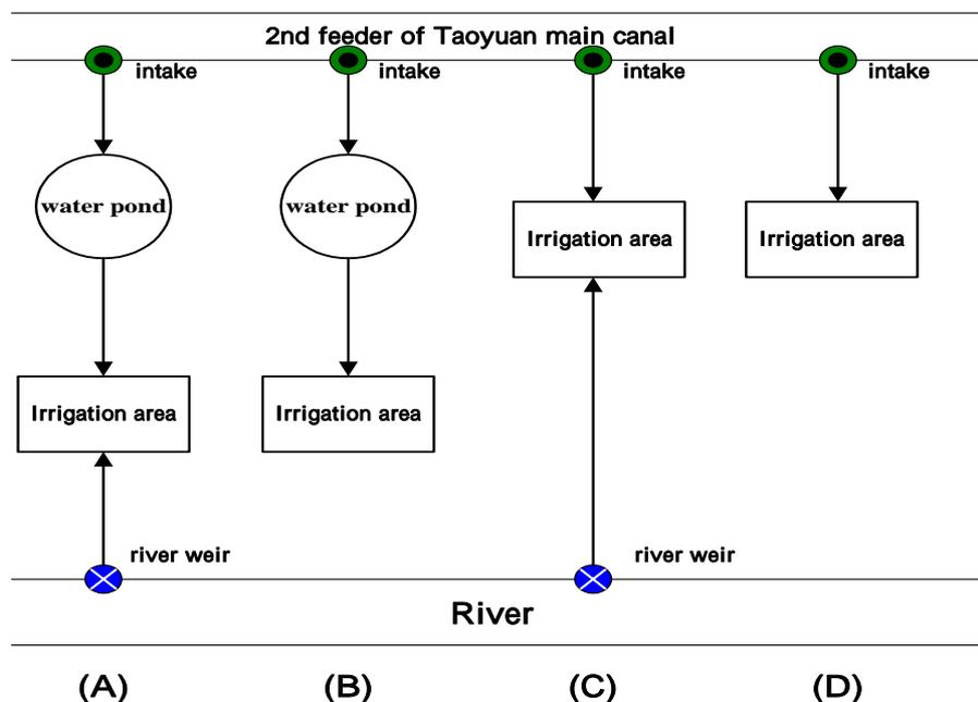
Figure 4. The diagram of supply style to irrigation area
