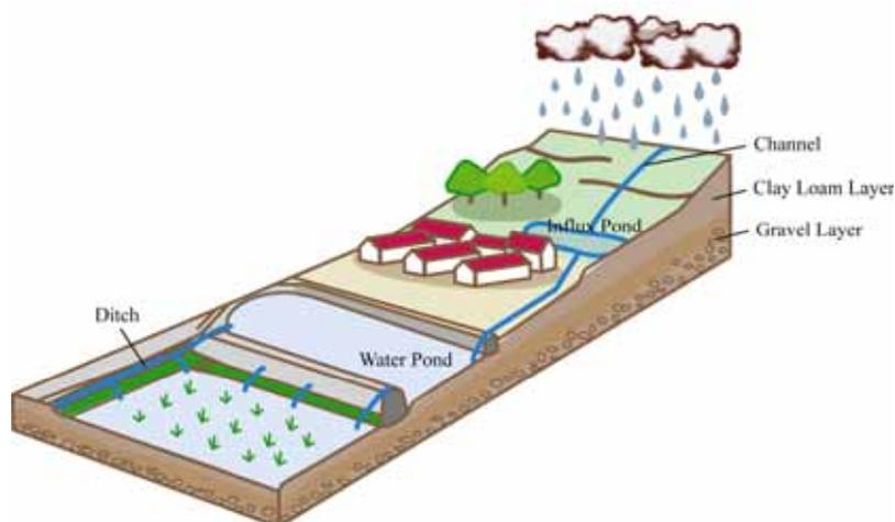
Figure2. Illustration of design theorem of water pond
